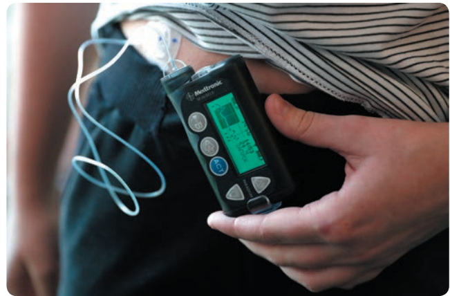
FIGURE 8.14 An insulin pump. The pump delivers a constant, small dose of insulin with a larger dose before meals or whenever the blood glucose level needs correcting
